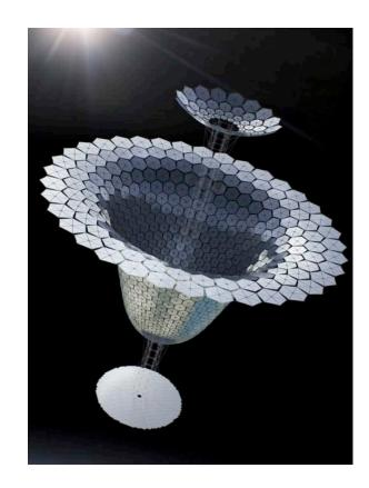
Each Alpha Mark IIIA is 9,800 tonnes (to GEO) - For output of 2 Gwatt continuous power
