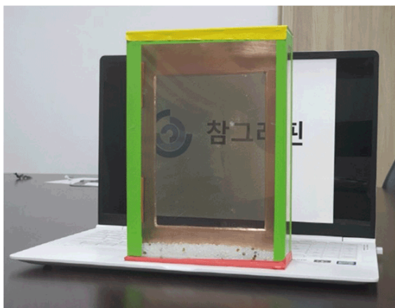
Extreme Ultra Violet light (EUV) pellicle reported to be made from dozens of layers of graphene Dimensions: 110 mm wide and a length of 144 mm Image Credit: Charmgraphene [1]
