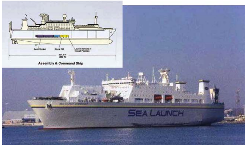
Fig. 11.1: Picture of the Sea Launch dedicated ship Sea Launch Commander used for transport of personnel, launcher, and supplies and for controlling the launch operations. A similar vessel would be valuable in the space elevator program for delivery of personnel, equipment and supplies.
